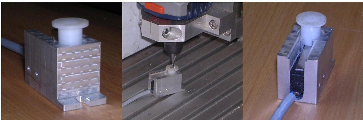
Figure 2: Example of a simple reference switch
