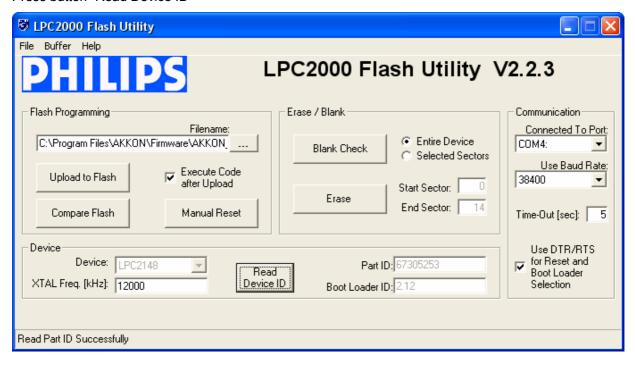
The Part ID and Boot Loader ID will appear in the exit boxes. Also the status of the operation is displayed in the status bar "Rear Part ID Successfully
