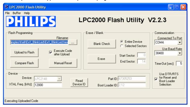
Select the application that should be uploaded to the Controller Board e.g. Ex1\_BlinkLed.hex and press button "Upload to Flash". After successful upload, the status bar should display the message "Executing Uploaded Code".
